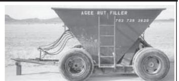
Wagon fills deep ruts with anything from crushed rock to soil. Material flows out of a hydraulically-operated door at bottom center.
