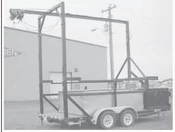
Trailer is used to prepare animals for butchering and then bring them back to a meat locker plant. Overhead trulley beam drops down for transport.
