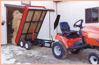
Trailer is dumped by a 3-ton, 30-in. hydraulic cylinder powered by a hand-cranked bottle jack. To dump load, Nolt simply pumps the handle (see arrow) on trailer tongue.
