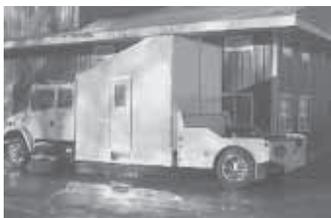
Custom-built RV tow vehicle has a storage compartment between cab and hitch (above). Hinged body swings out to unload motorcycle without unhitching RV (below).
