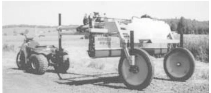
**Power Roll's hydraulic-powered rotating rollers aggressively apply chemical to tall-growing weeds.**
