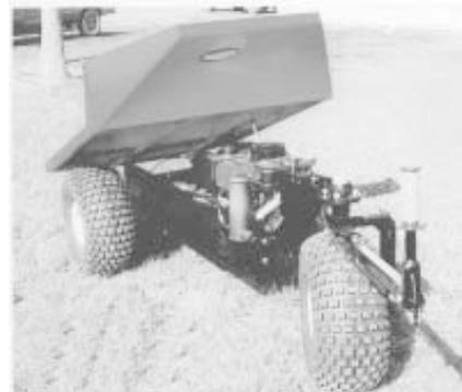
**Walk-behind hand truck carries up to 1,000 lbs. of cargo and is controlled by a handle on front.**
