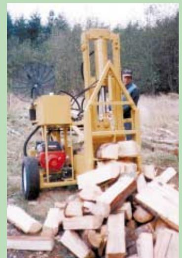
Splitting blades are adjustable to make 2 or 4 pieces. An 8-way splitter attachment is optional.
