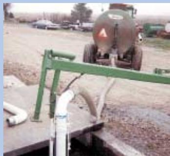
To fill a tank, elbow pipe is replaced by a hose. Homemade pump is so powerful Winters says he doesn't have to use vacuum to fill tank.
