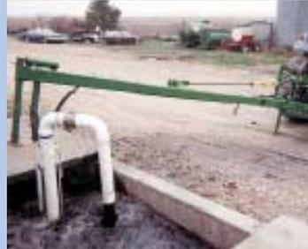
To stir up pit, elbow pipe is attached to top of agitator-pump and material is pumped back into pit.
