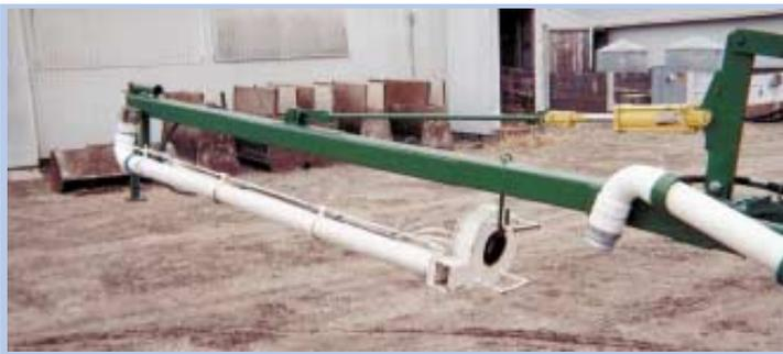
Agitator folds up flat for transport. Elbow pipe hangs on bracket behind tractor.
