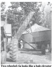
Two-wheeled rig looks like a bale elevator instead of a chain and apron that has a steel catwalk.
