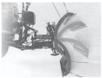
A hydraulic cylinder is used to fold top 3/4 of blade forward 180 degrees. A joystick control in cab is used to rotate blade.
