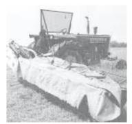
To protect himself from flying objects, Cranfil made an expanded metal screen and bolted it to his tractor fender.
