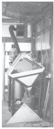
Stripped-down washing machine case was set on its side at a 35 degree angle. Graham used galvanized sheet metal to close off the top and bottom, leaving a large access door for easy maintenance.
