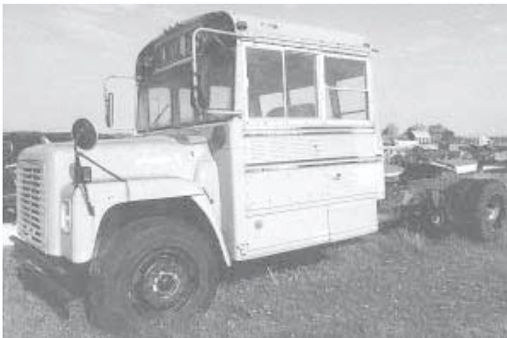
Scripter cut down a school bus and mounted a semi fifth wheel hitch and plate on back. He uses bus to pull his 23-bale hay trailer.
