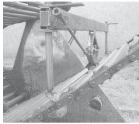
Tool consists of a screw jack operated by an impact gun. It can be used to straighten slats right in the baler.
