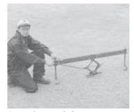
Automotive screw jack mounts at center of 5-ft. length of 2 by 3-in. steel tubing. the outer arms. Now, with the 12-in. throat, the screw jack is past half-way before it starts to push on the chain slat."
