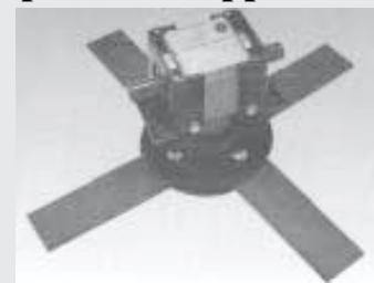
with a field cultivator. My soybeans averaged about 50 bu. per acre this year so the system is working for me. My only maintenance cost was to replace a gearbox that got damaged by a rock. I use an offset grinder to keep the blades sharp. The blades are reversible. A set of blades can be expected to last about four years.
