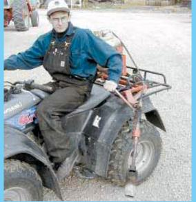
Outrigger arm makes it easy for driver to swing propane torch in or out, forward or back.
