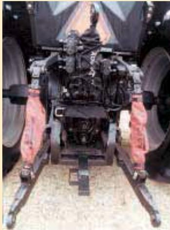
**Waterproof covers have a velcro patch at each end, allowing sleeve to be drawn tightly up against threaded part of link.**
