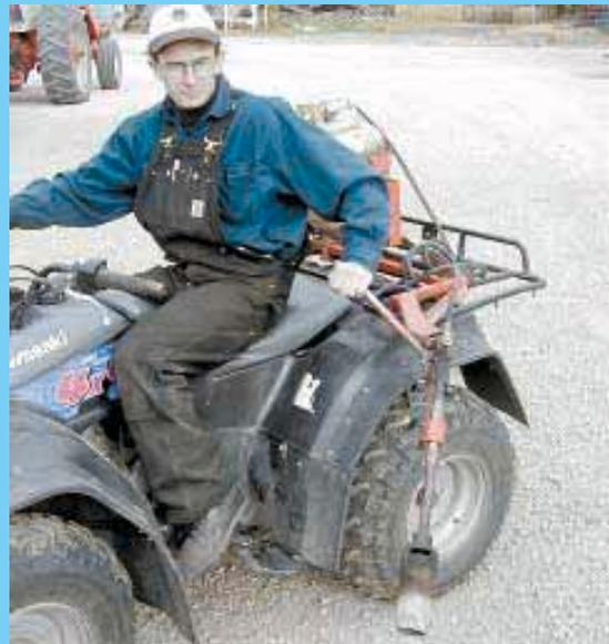
**Outtrigger arm makes it easy for driver to swing propane torch in or out, forward or back.**
