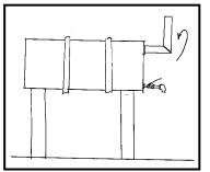
of 2-in. pipe formed into a 90° elbow. Screw one end into the 2-in. hole, swinging it up to fill and down for a rain-proof vent. A 3/4in. ball valve installed in the lower 3/4-in. tapped hole is used to draw off the oil."
