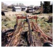
Rake folds in for transport. Two wheels from an old harrow bar serve as front transport wheels.
