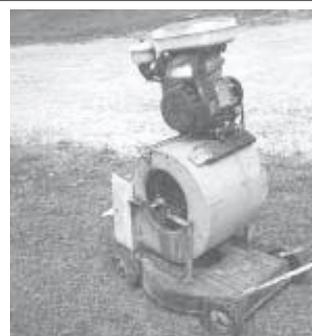
Engine belt-drives the fan. Wood sideboards direct air flow downward.
