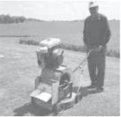
Sexton mounted an old house furnace fan on top of a push-type lawn mower deck, then bolted a gas engine on top of fan.
