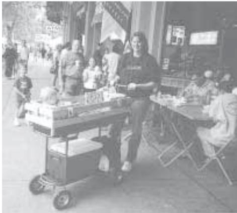
Voth's home-built baby carriage is based on a 4-wheel cart with a "stretched" red wagon box mounted above.
