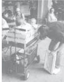
Steering handle controls tie rods that connect to front wheels.
