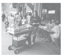
Voth's home-built baby carriage is based on a 4-wheel cart with 'stretched" red wagon box mounted above.
