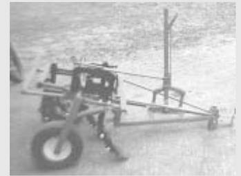
**Schueller pulls his home-built mini chisel plow behind his Deere garden tractor. It rides on a pair of 8-in. high wheels and is equipped with five shanks that dig a path 2 1/2 ft. wide.**
