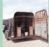
Inside trailer's back door Ruby installed a gate made from a cattle panel. Two narrow wooden doors built into gate can be raised to allow dogs to leave trailer for exercise.
