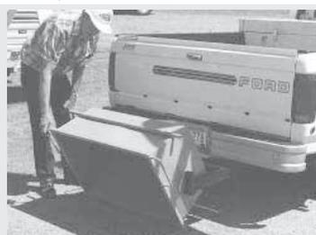
Box empties completely when dumped. No need to lift loads into pickup bed.
