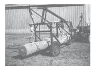
Reeks's log hauler straddles the log. Two sets of hand-powered log tongs lift it. on the highway.
