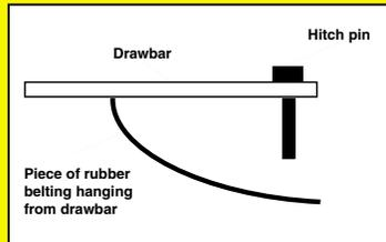
Here's a very simple idea to keep hay and other crop residue from catching on hitch pins. Just hang a small piece of rubber belting from the drawbar ahead of the hitch pin. You'll never lose another hitch pin.
