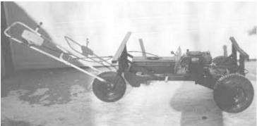
Self-propelled boat mover was built from a stripped-down Deere riding mower. It's powered by the mower's 3 1/2-hp, 2-cycle engine.
