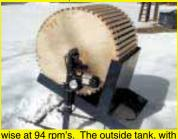
wise at 94 rpm's. The outside tank, with the slats, runs 12 to 14 rpm's. I can shell a peck of nuts in anywhere from 5 to 9 min., depending on the thickness of the shell. It works great. I have shelled 80 bu. in 4 weeks. About 90 percent of the nuts come out in halves. I am applying for a patent on this great new design. (Hoover A. Lingle, 1022 S. Main GQ St., Salisbury, N.C. 28146 ph 704 279-2465)
