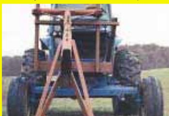
to lift the rack up by the top ring and lower it over the bale without ever leaving the tractor seat. Here are some photos that show how the boom can be mounted on front of my Ford 7700 2-WD tractor, allowing me to haul the feeder and carry a bale on back at the same time. The boom is offset to the right side of the tractor so I can see the end of the boom
