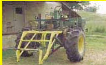
the arms. A hydraulic cylinder mounted behind the frame is used to move the bale up or down and to tilt the bucket.
