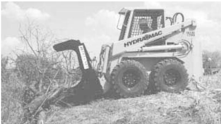
**New grapple bucket is designed to scoop up brush, rocks, and other debris but leave the dirt in place. Bucket is available with or without a grapple.**
