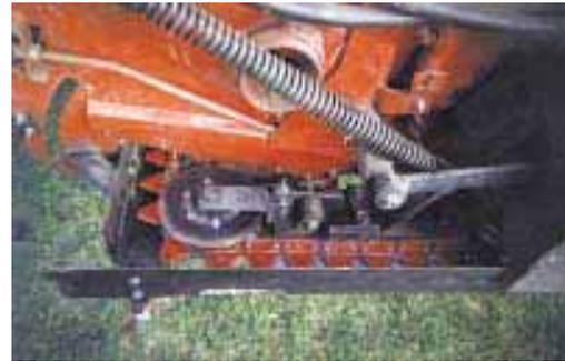
Continuous 50-ft. long cutter chain is equipped with replaceable sickle sections. As chain rotates, it returns through a trough under platform.
