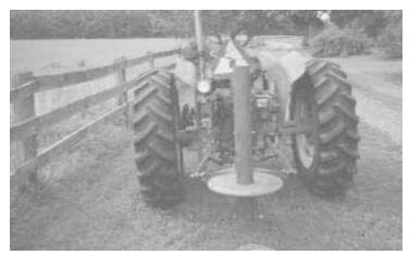
The 3-pt. mounted wire unroller is made from a piece of 4-in. dia. pipe and two 20-in. round steel plates - one bolted down and one left free to turn with the wire as the tractor goes along.
