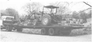
With rack removed the flatbed trailer can be used to haul conventional loads.
