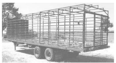
Rack will hold 18 to 20 head. When not in use for hauling cattle, rack is simply stored on the ground out of the way.
