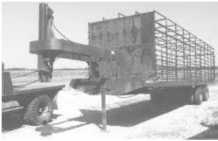
"Convertible" flatbed trailer can be fitted with an 8 by 30-ft. cattle-hauling rack that's winched into place on the trailer bed.
