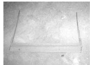
metal bender that lets me bend sheets of metal at a 90 degree angle. It's equipped with a hinged handle on each side. I place the bender in a vise with the handles straight up in the air. Then I slip the metal sheet in under a bar and use a pair of vise grips to keep the sheet in place. To make the bend I simply pull both handles back toward me. I copied it off a photo of a commercial unit. It makes a nice clean 90 bend."
