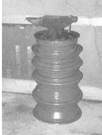
16-in. dia. wheel rims on top of each other, with one 14-in. wheel on top. All are welded together. Then I bolted an anvil to the top. Makes a solid, heavy stand that will take all the pounding you can dish out yet you can also roll it around the shop, if necessary."
