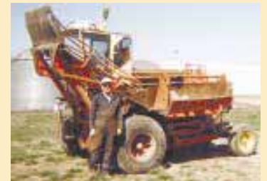
Bucket tilts up and back to dump rocks into a box off an old gravel truck.
