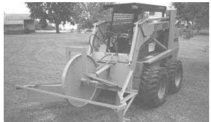
Shop-built 4-ft. long V-blades are angled to cover a total area of 6 ft.
