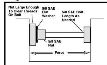
**Floyd Stivers, Stroud, Okla.:** Floyd says a common problem on small block Chevrolet V-8 engines from the late 1960's through the early 1980's is this: The heat from the engine causes the cast iron exhaust manifolds to "draw up" so much that bolts cannot be started in the original holes when reinstalling them.
