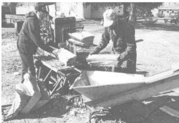
Hydraulic-powered platform lifts logs onto splitter table.
