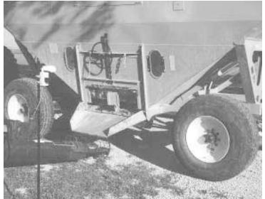
Electronic eye "reads" light reflected from tape on side of wagon or truck, turning on bulb to alert driver.
