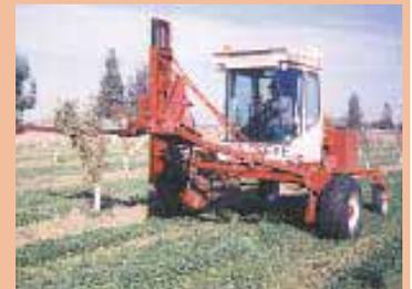
Tree-trimming attachment was built by mounting a swather sicklebar on an old forklift mast. It reaches up to 12 ft. high.
