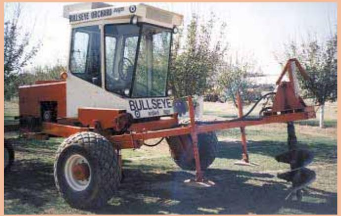
Alberico mounted a 9-ft. long steel A-frame on front of a 1970's Hesston 6400 swather, then mounted hydraulic-driven auger on end of A-frame.
