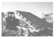
Trailer's tandem axle follow the ground contour and keep the wagon from sinking into soft ground.
