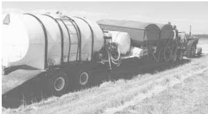
Broaddus's 52-ft. long drop deck semi trailer carries everything he needs for planting and spraying. The bed is lower than a standard flatbed so it's easier to get up on.
