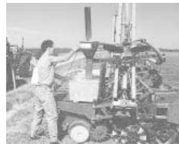
A “Bean Hustler” pneumatic conveyor is used to deliver soybean seed from gravity boxes on the trailer to row units on Broaddus's 12-row Deere planter.
