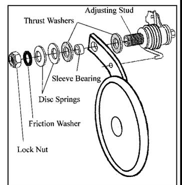
**Force of approximately 350 lbs. is applied through two disc springs.**
