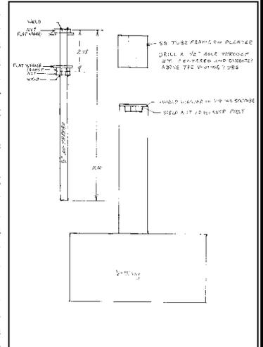
**Screw-type adjustment for V-wings.**
