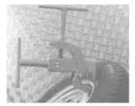
Tool works with two hand cranks that force the bead off the rim.
