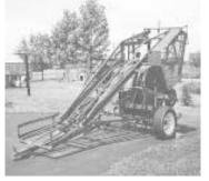
Unit is also available as a hydraulicallyoperated model on wheels that automatically lays down a Zimmie stack.
