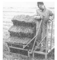
On the manual stacking unit, a person rides along on the unit to stack the bales and release them onto the ground.
