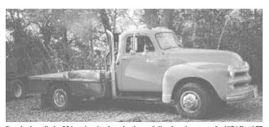
Draehn installed a 256 cu. in., 4-cyl. turbocharged diesel engine - out of a 1976 Ford 77 tractor - in this 1954 Chevy S4 1 1/2-ton pickup. "It really has pulling power," he says.
