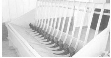
Electric-powered hair remover consists of a 10-ft, long steel tub with a powered shaft at bottom that's fitted with rubber flaps. Animal is lowered to bottom of tub by a steel cradle with rods spaced 3 in. apart. The rubber flaps come up through the bars on the cradle to remove the hair.
