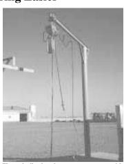
Home-built slaughter system starts with this 15-ft. high electric-powered hoist equipped with a 10-ft. long arm on top that's free to rotate 360 degrees. Hoist rolls back and forth on arm.
