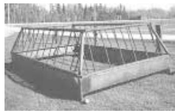
Skid-mounted silage or hay feeder made out of same thick-walled oilfield pipe.
