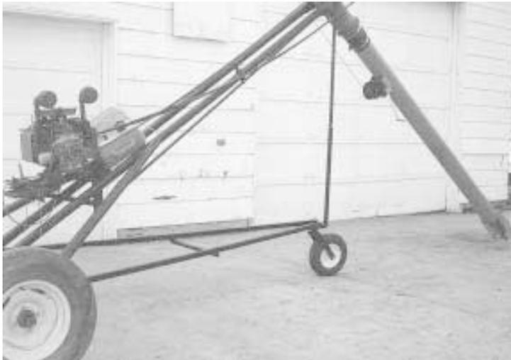
Mover consists of an 8-in. dia. pneumatic wheelbarrow wheel that castors on a triangular frame attached to the auger axle.
