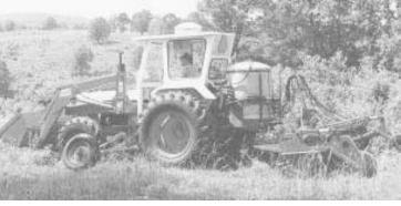
"Roll-On Applicator" consists of a 10-ft. wide bark scraper followed by an 18-in. dia. herbicide applicator drum.
