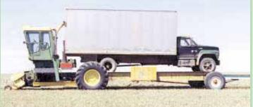
Forage harvester's spout actually extends inside the truck. Note big flotation tires on front of trailer and hydraulic-operated dovetail ramp on back.
