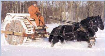
Homemade "snow packer" creates a 6-ft. wide trail for sleighs. It was made out of a 6-ft. wide, discarded wire reel from a utility company.
