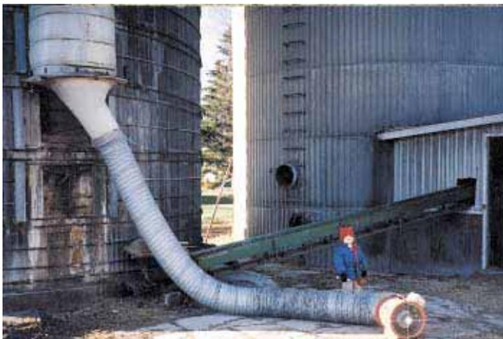
High-speed aeration fan pulls poisonous gases out of silo through chute before workers enter. It can be moved from silo to silo, as needed.
