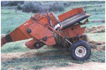
Inverter was made out of an IH 2400 round baler. Two hydraulic cylinders raise the machine, providing up to 2 ft. of ground clearance to easily pass over end windrows.
