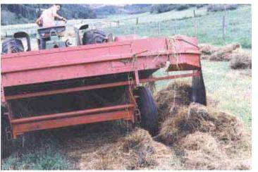
Hay comes around the corner of the horizontal belt and onto the outfeed chute. Inverter handles windrows up to 5 ft. wide.
