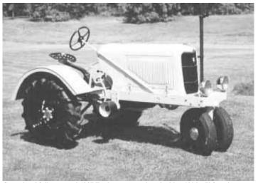
Cummings' fully restored 1937 Ford tractor, equipped with a 100 hp V-8 engine.
