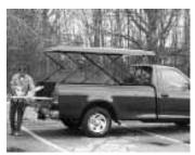
The scissors lift fiberglass cover can be stopped at any height up to 6 1/2 ft., allowing you to use it as a covered work area.
